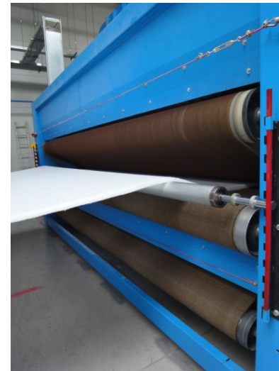
Photo 7-8: Made-to-measure dryer belt from GKD meets the special requirements of the thick insulation products.
