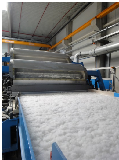
Photo 4: Fine fibre opening
