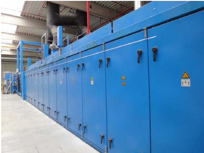
Photo 9: 14-metre-long double-belt oven
