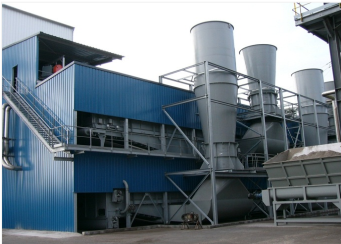
Picture 3: Low temperature belt dryers with woven mesh process belts manufactured by GKD reduce the energy consumption of the beet pulp drying process.
