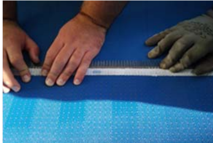
Picture 6: The patented GKD PAD seam connects the ends of the endless process belt.
