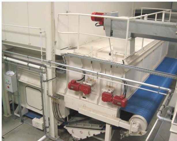
Picture 7: In spite of their small mesh aperture, the Conducto® 5065 belts are extremely air permeable.
